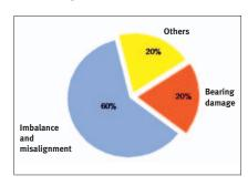
During operation, imbalance can generate considerable vibrations that lead to secondary damage such as premature bearing wear or fatigue fractures.
